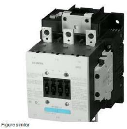
CONTACTOR, 90KW/400V/AC-3, AC(40...60HZ)/DC OPERATION UC 200...277V AUXIL. CONTACTS 2NO+2NC 3-POLE, SIZE S6 BAR CONNECTIONS ELECTRONIC OPERATING MECHANISM WITH 24V DC PLC INTERFACE SCREW TERMINAL
